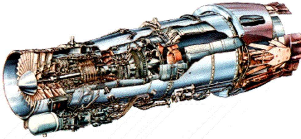
**Figure 3: Schematic Of 1970s Technology Gas Turbine**
