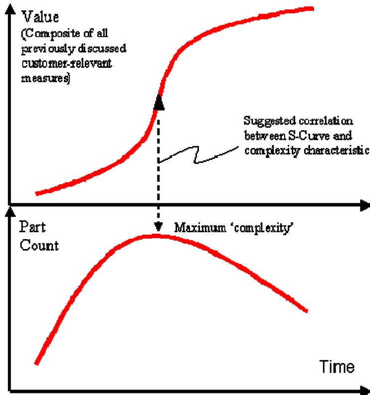
Figure 6: Suggested Relationship Between Expansion-Convolution Transition and System Part-Count
