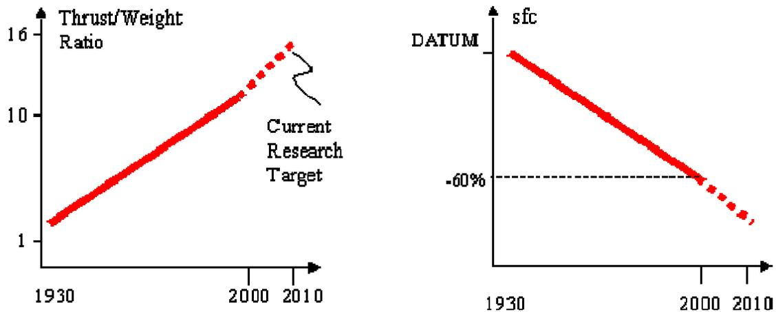
**Figure 1: Improvements in Gas-Turbine Mean T/W And sfc As A Function Of Time**
