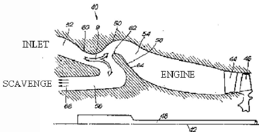
**Figure 7: US Patent 5,139,545 Particle Separator**
