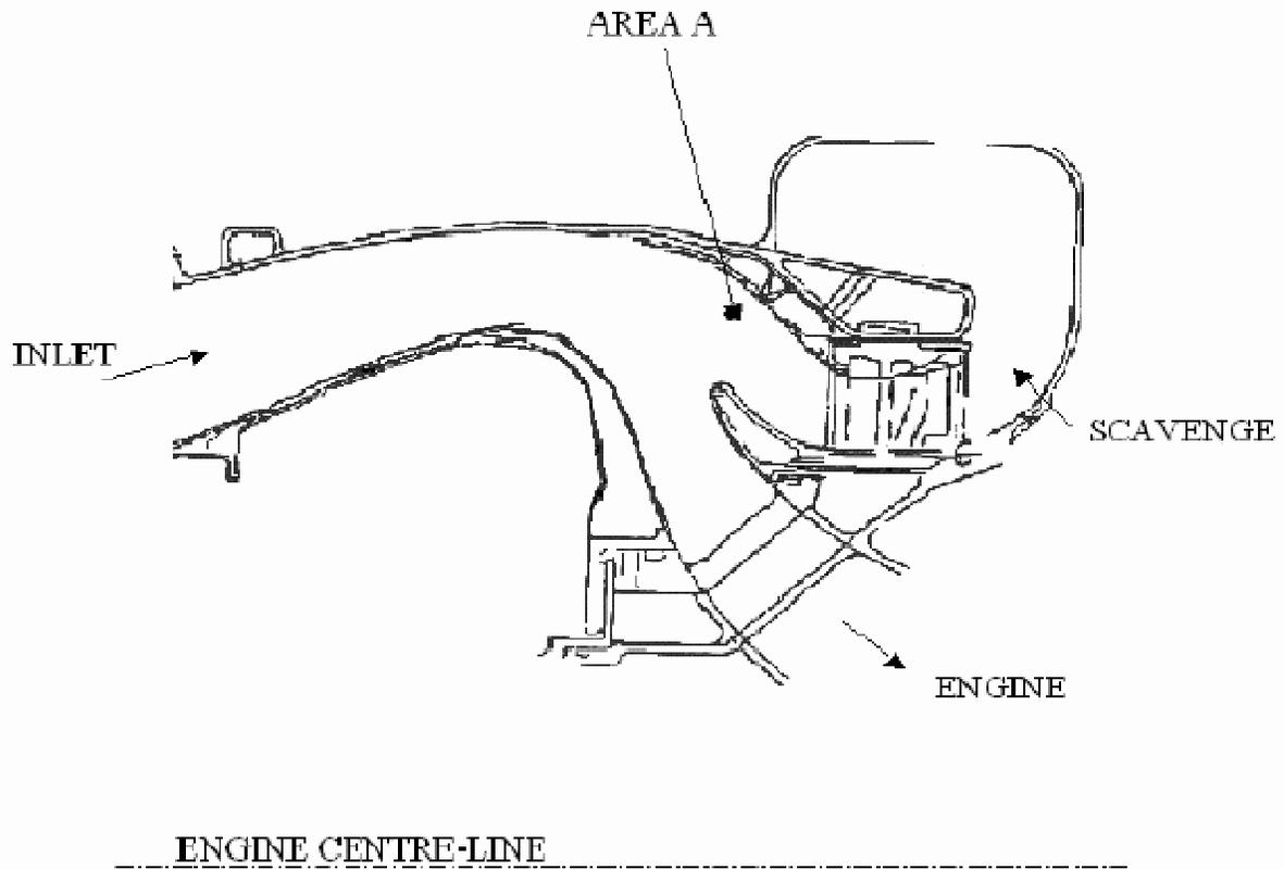
**Figure 6: Typical Engine Mounted Particle Separator**
