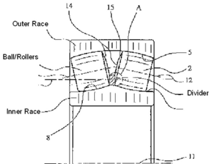
**Figure 3: Exemplar State Of The Art Bearing System.**
