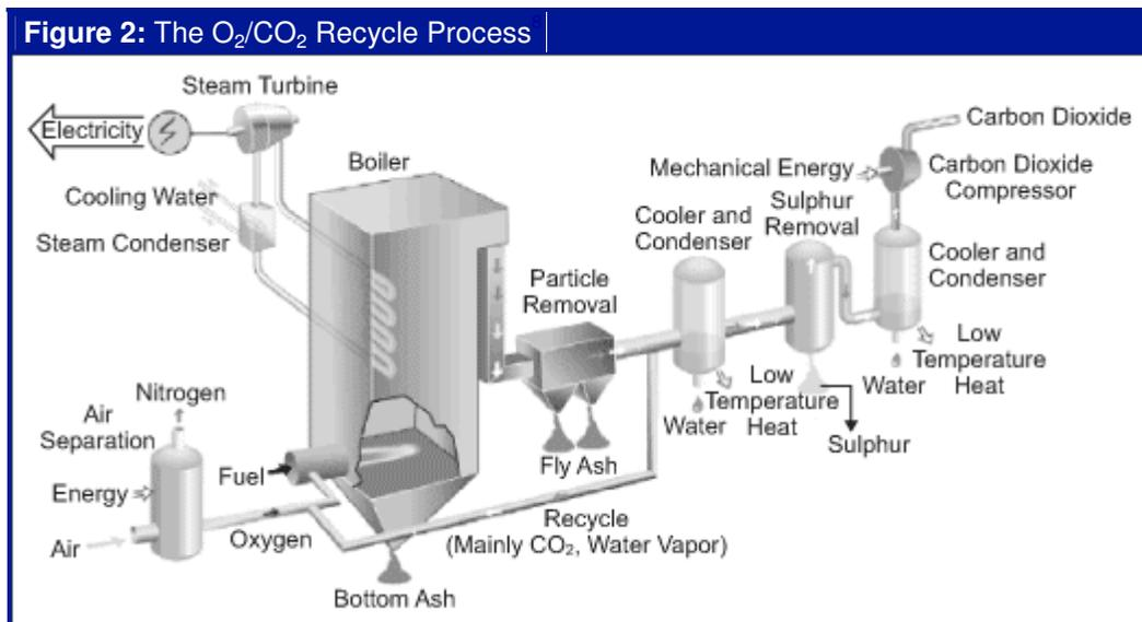
The reported challenges involved with the O<sub>2</sub>/CO<sub>2</sub> recycle approach relate to individual process efficiencies that contribute to the overall efficiency of power generation. Current research is
