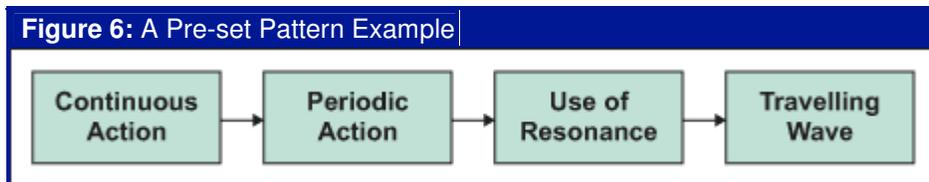
A look at the vanadium membrane patents in the U.S. patent database reveals that the current designs are at the first stage of this progression, "continuous action." Should the ultrasonic vibration idea turn out to be practically viable, then the system will make the predicted jump to the second or third stage of the trend.
