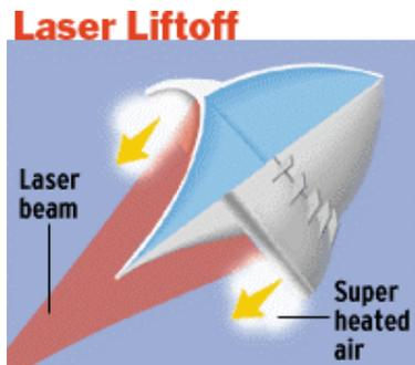
In simple terms the system works by firing a laser at a strategically shaped forebody – see Figure below – and using the heat generated by focusing the laser energy to heat air (an existing resource in the system!) which then expands out of the rear of the craft to provide thrust. Essentially the system achieves a much higher payload fraction because the atmospheric air is the propellant.
