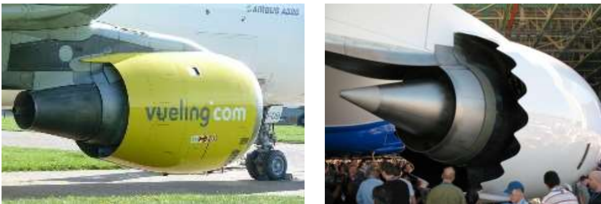
Figure 1: ‘Conventional’ Versus Fluted Engine Nacelle
