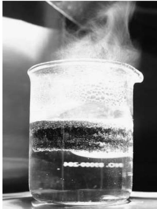
As sun heats the graphite, it creates a pressure difference that pulls water up through the foam pores, like a sponge. When the water hits the graphite hot spot, it turns into steam. The scientists report that this inexpensive system reaches 85 percent efficiency in converting the solar energy into steam. The study was published in journal Nature Communications this month. [Hadi Ghasemi et al, Solar steam generation by heat localization:
