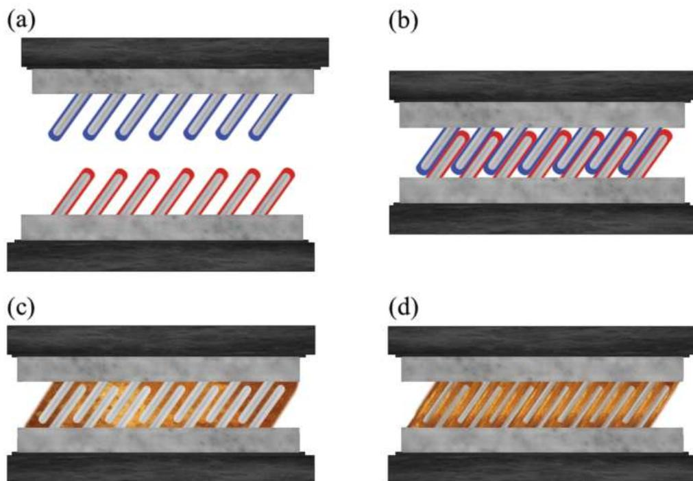
a) Coated rods are arranged along a substrate, like angled teeth on a comb. b) The teeth are then interlaced. c) When indium and gallium come into contact, they form a liquid. d) The metal core of the rods turns that liquid into a solid. The resulting glue provides the strength and thermal/electrical conductance of a metal bond.
