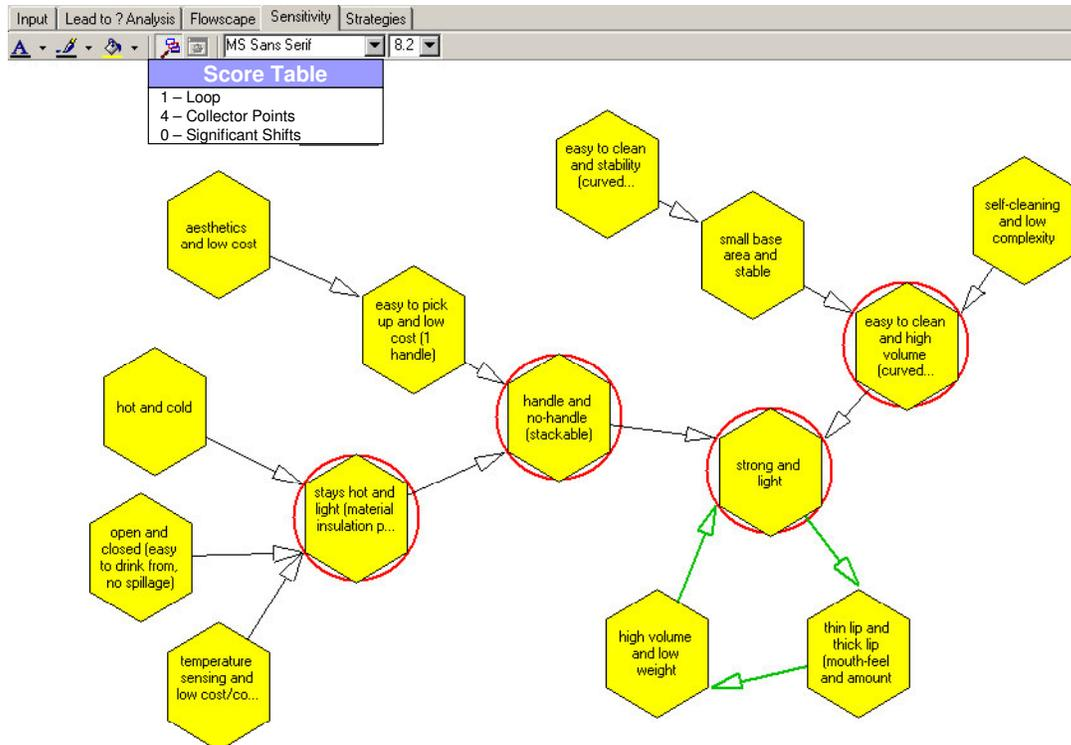
**Figure 3: Sensitivity Analysis Performed By Perception Mapping Software Tool**
