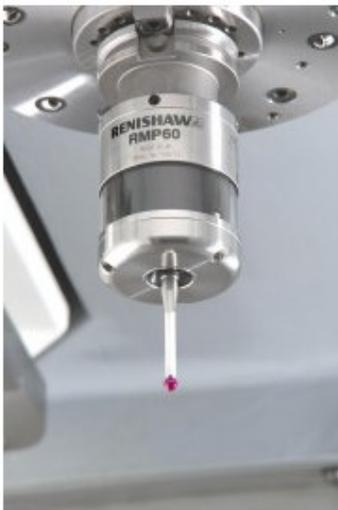
*Radio probe systems allow for great flexibility in the positioning and orientation of the receiver, particularly where line-of-sight restrictions make optical transmission systems impractical. The RMI is a combined antenna and interface so no separate enclosure is required to be mounted in the control cabinet. Conduit routings are therefore simplified for faster installation, making the RMP60 highly suitable for retrofitting to existing machines.*
