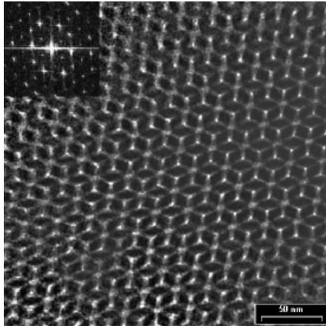
**Transmission electron micrograph of the cubic structure of the new hybrid material showing pores about 10 nanometers across.**
