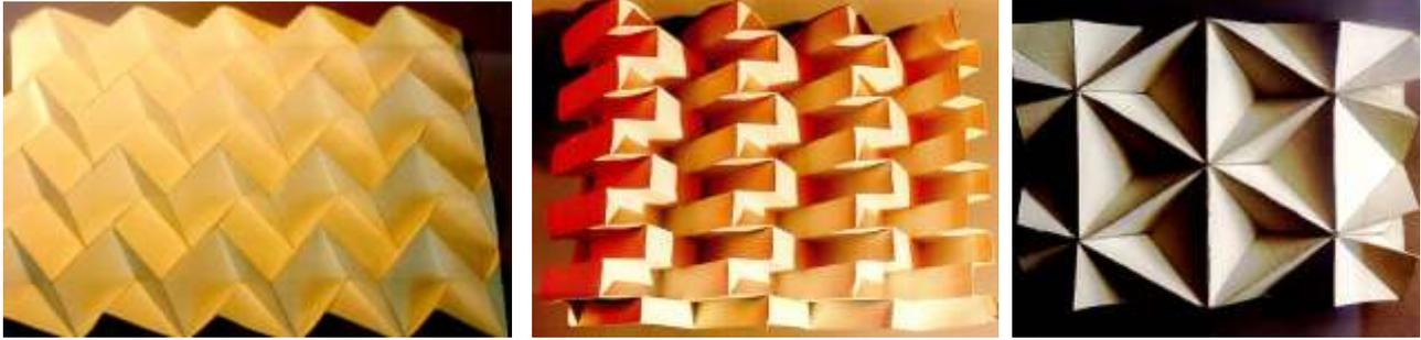
Doubly periodic folded (DPF) sheet is stronger than corrugated construction and has potential applications in aerospace for structures, cars for impact absorption and lighter weight and more effective packaging.
